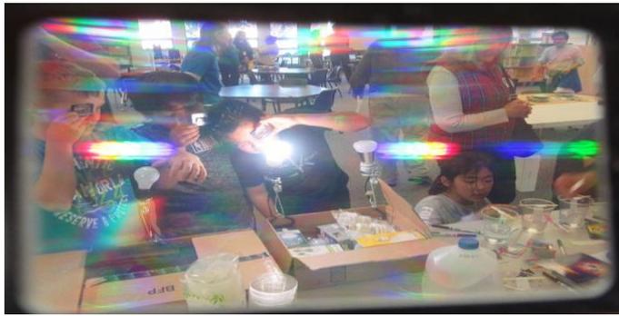
*The view through the diffraction grating looking at the compact fluorescent light bulb. Notice how the white light is divided into red, orange-yellow, green and blue light bulbs.*
